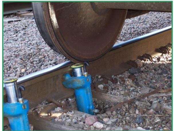
As with all piston type retarders, energy extraction is speed related. Thus, higher railcar speed equals higher energy extraction. When a retarder setting is given as, for example, 4mph – 1180J, this means that at 4mph this retarder will extract 1180 Joules of energy from the railcar. As energy cannot be destroyed, but transferred from one form to another, and from one body to another, the extracted energy is transformed into different energy forms, such as heat, sound, vibration, etc.
